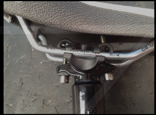
Tighten bolts to get desired seat angle.
