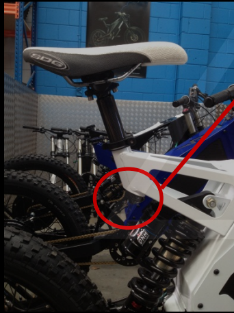
Loosen rear bolt
