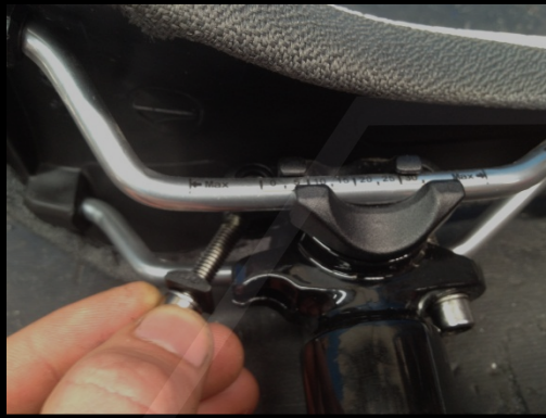
Fit clamp to seat rails.
