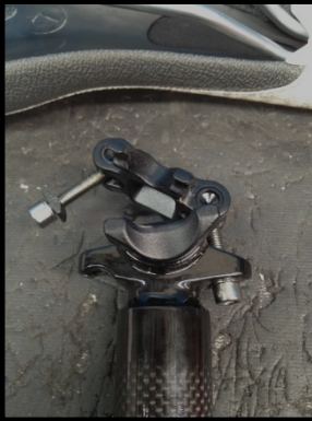
Loosen rear bolt
