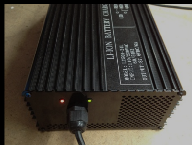
A red and green light is displayed when charger is disconnected from bike or battery is fully charged
